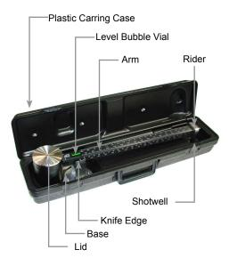
Metal Mud Balance Complete with Carrying Case 4-Scale: #115-00
