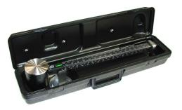
Metal Mud Balance (Machined Balance)
